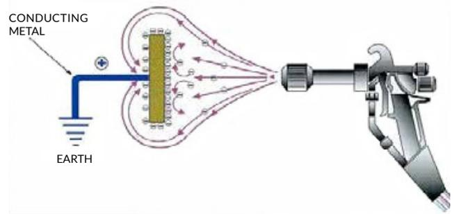
Due to their high conductivity, water-based coatings can be used in these electrostatic applications, but only with special application techniques. The system, suitable for spraying water-soluble products and therefore safe for the user, complete with a spray gun (usually airmix but also airless) and generator, offers the following advantages:
