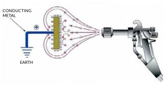
Due to their high conductivity, water-based coatings can be used in these electrostatic applications, but only with special application techniques. The system, suitable for spraying water-soluble products and therefore safe for the user, complete with a spray gun (usually airmix but also airless) and generator, offers the following advantages: - excellent all-over coverage of the workpiece;
